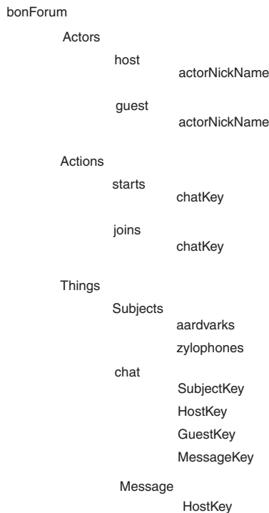
Figure 5.4 Designing bonForum XML using a tree diagram.
